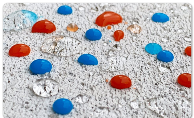
Water and dirt repellency on hydrophobized aerated concrete
