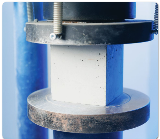
Compressive strength testing of concrete specimens
